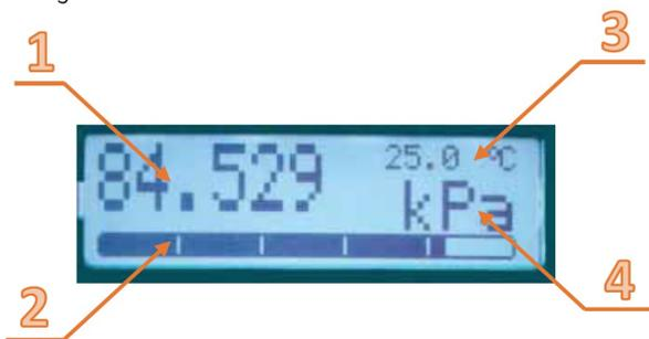
Picture shows main view of standard display mode "Reading display" screen.
